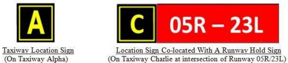
Figure 4.3. (Added-WRIGHTPATTERSONAFB) Typical Location Signs.
