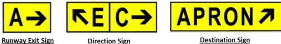
Figure 4.2. (Added-WRIGHTPATTERSONAFB) Typical Direction Signs.
