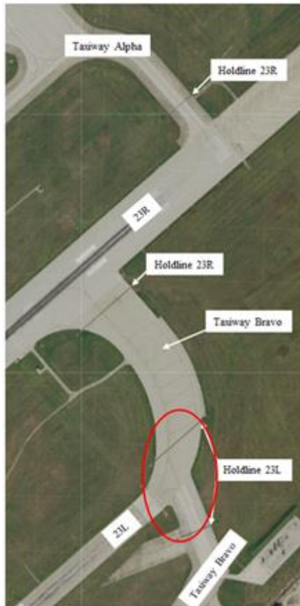
Figure 4.19. (Added-WRIGHTPATTERSONAFB) Hot Spots.
