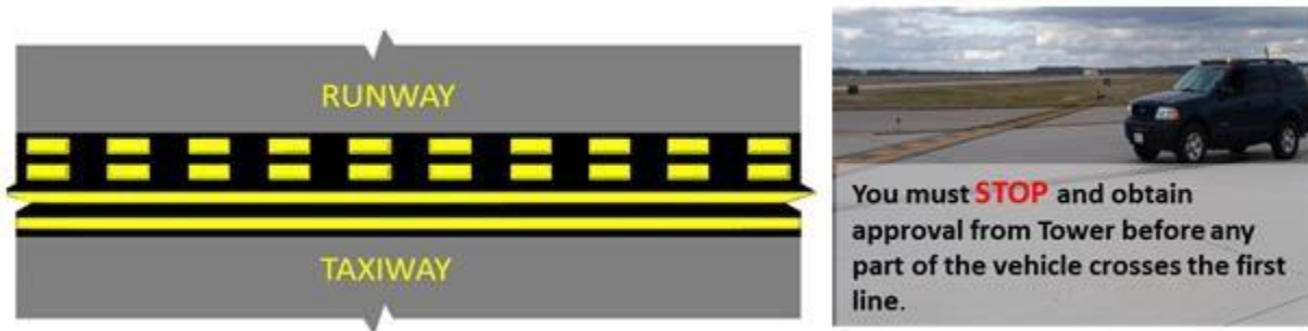
Figure 4.8. (Added-WRIGHTPATTERSONAFB) Typical Runway Hold Position Marking Co-located With Runway Hold Sign.
