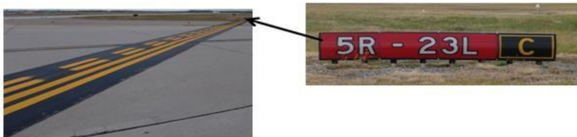
Figure 4.8. (Added-WRIGHTPATTERSONAFB) Typical Runway Hold Position Marking Co-located With Runway Hold Sign.
