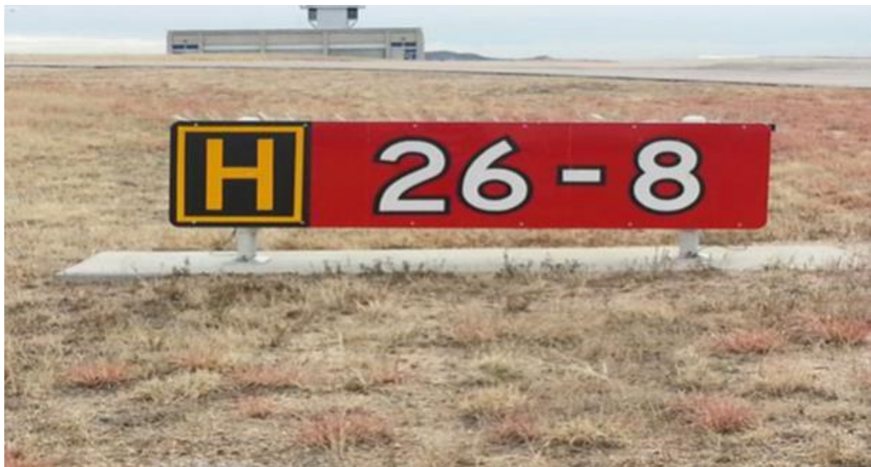
Figure A11.10. (Added-USAFA) Mandatory Runway Hold Position Sign with Taxiway Location Sign.
