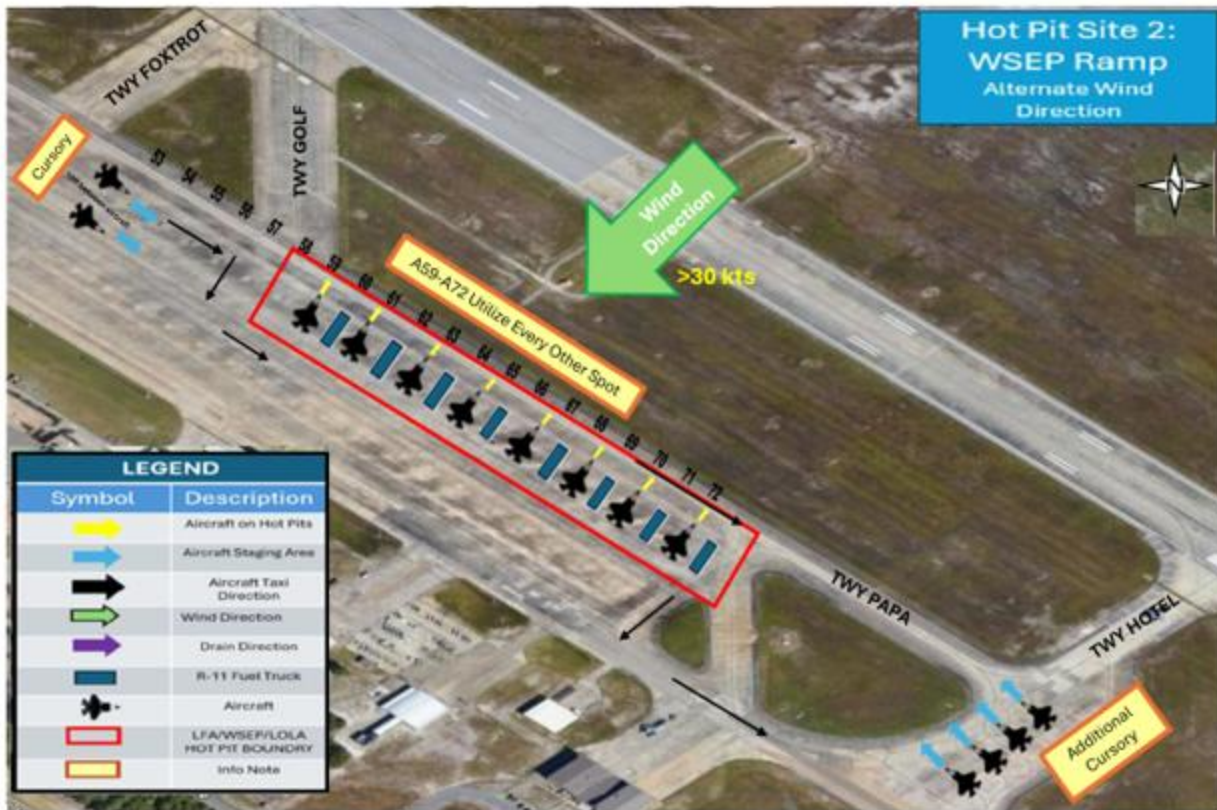
Figure 1.4. Site #2 East/WSEP Ramp Hot Pit Alternate Flow.
