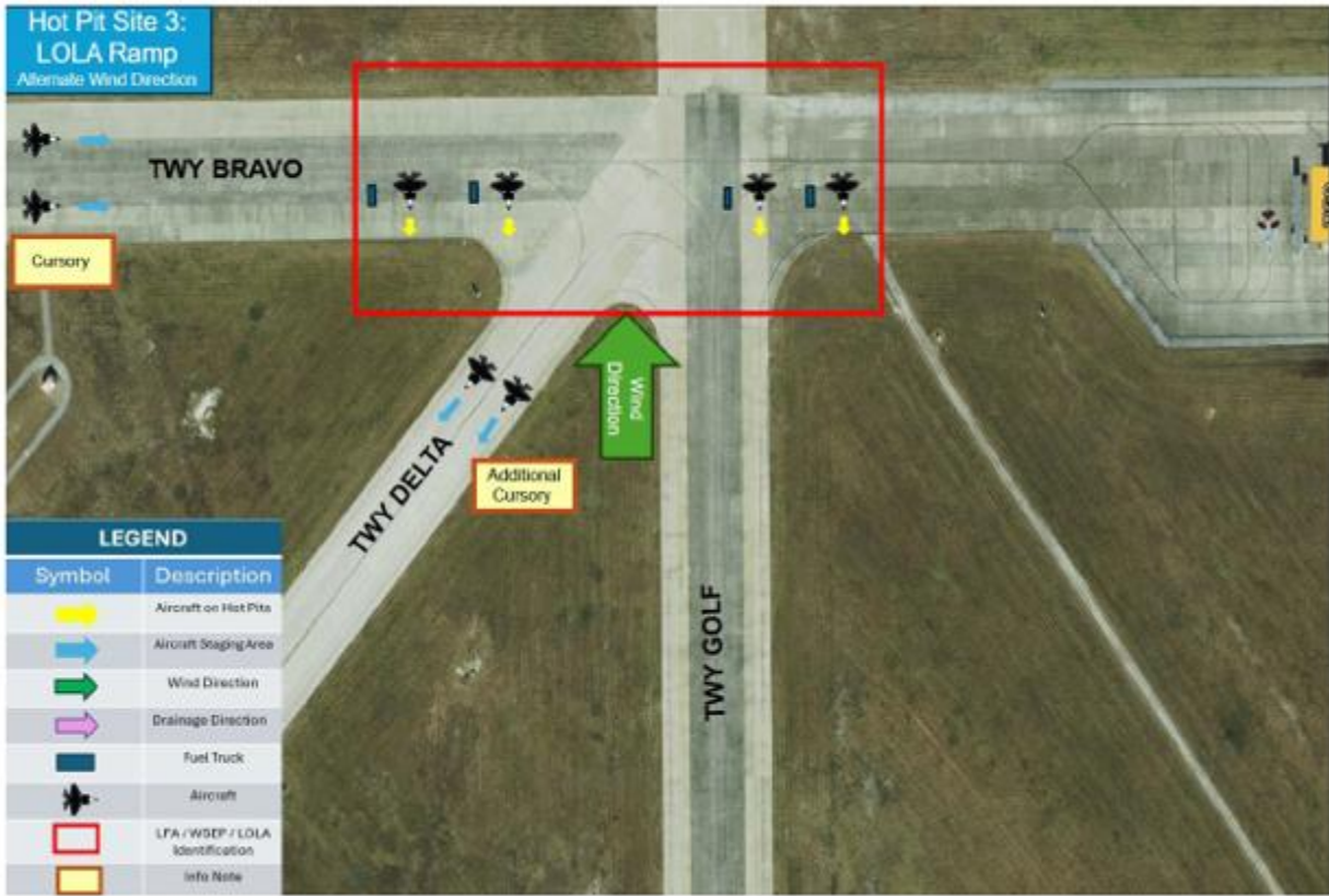
Figure 1.7. Site #3 B-D-G Hot Pit Alternate Flow.
