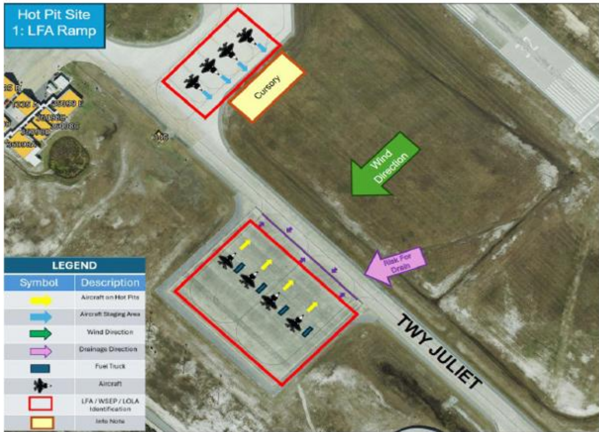
Figure 1.1. Site #1 LFA Ramp Hot Pit Flow.
