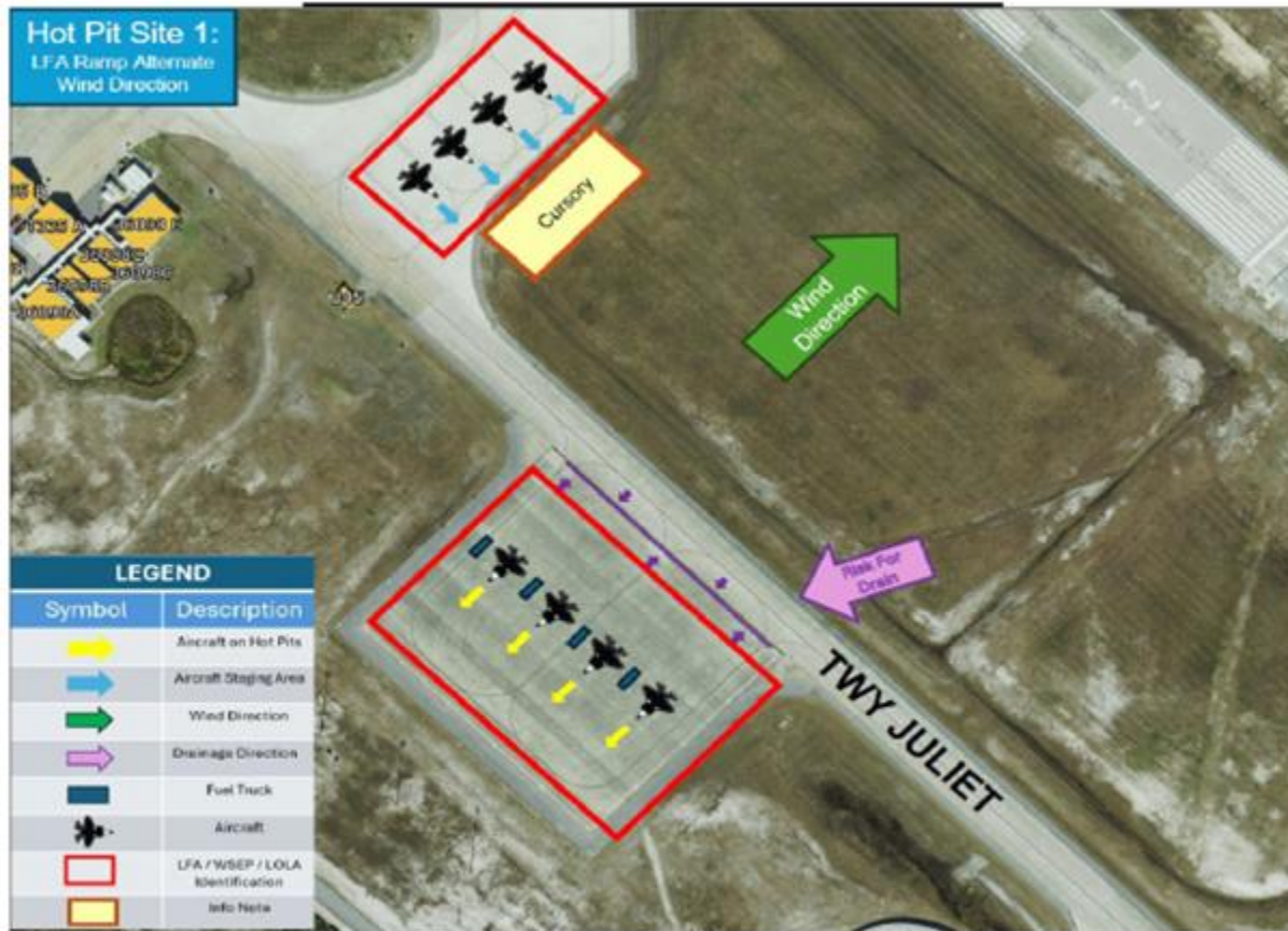
Figure 1.2. Site#1 LFA Ramp Hot Pit Alternate Wind Direction.
