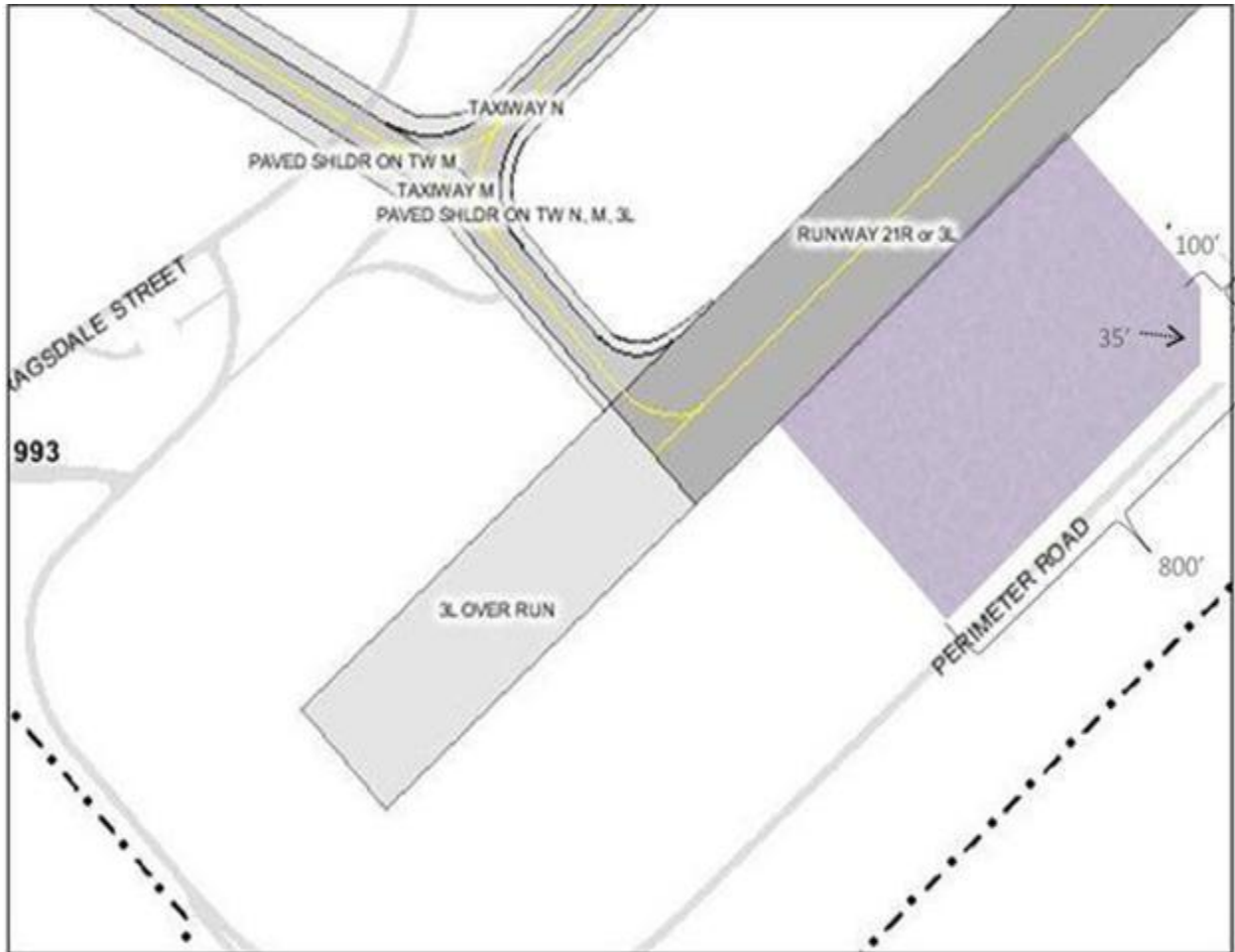
Figure A14.1. Runway 03L Glideslope Critical Area.
