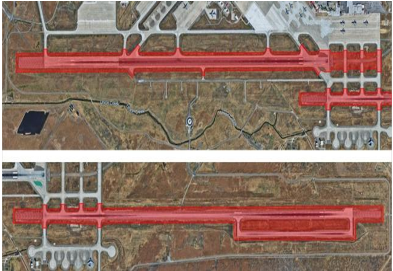
Figure A2.1. Controlled Movement Area.
