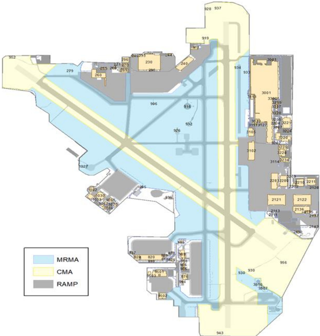
Figure A6.1. Runway/Taxiway System, Controlled Movement Area (CMA) and Mandatory Radio Monitor Area (MRMA).
