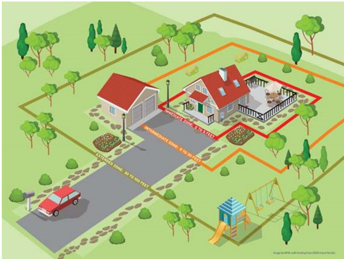
Figure 3.1. Ignition Zone Clearances.
