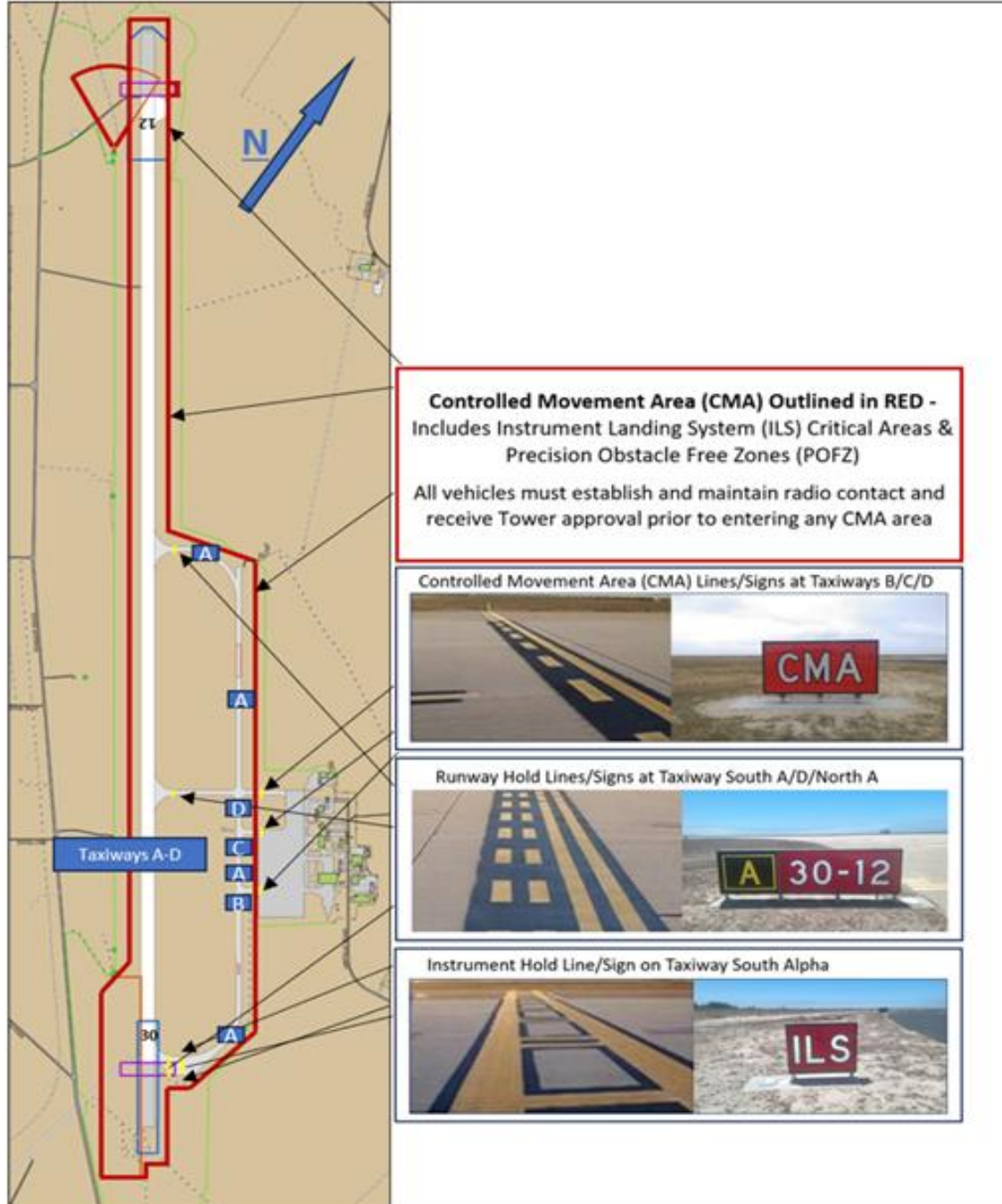
Figure A4.1. Controlled Movement Area.
