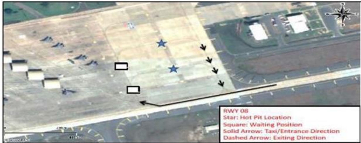
Figure 2.4. Hot Pit Refueling RWY 08 Hot Pits.
