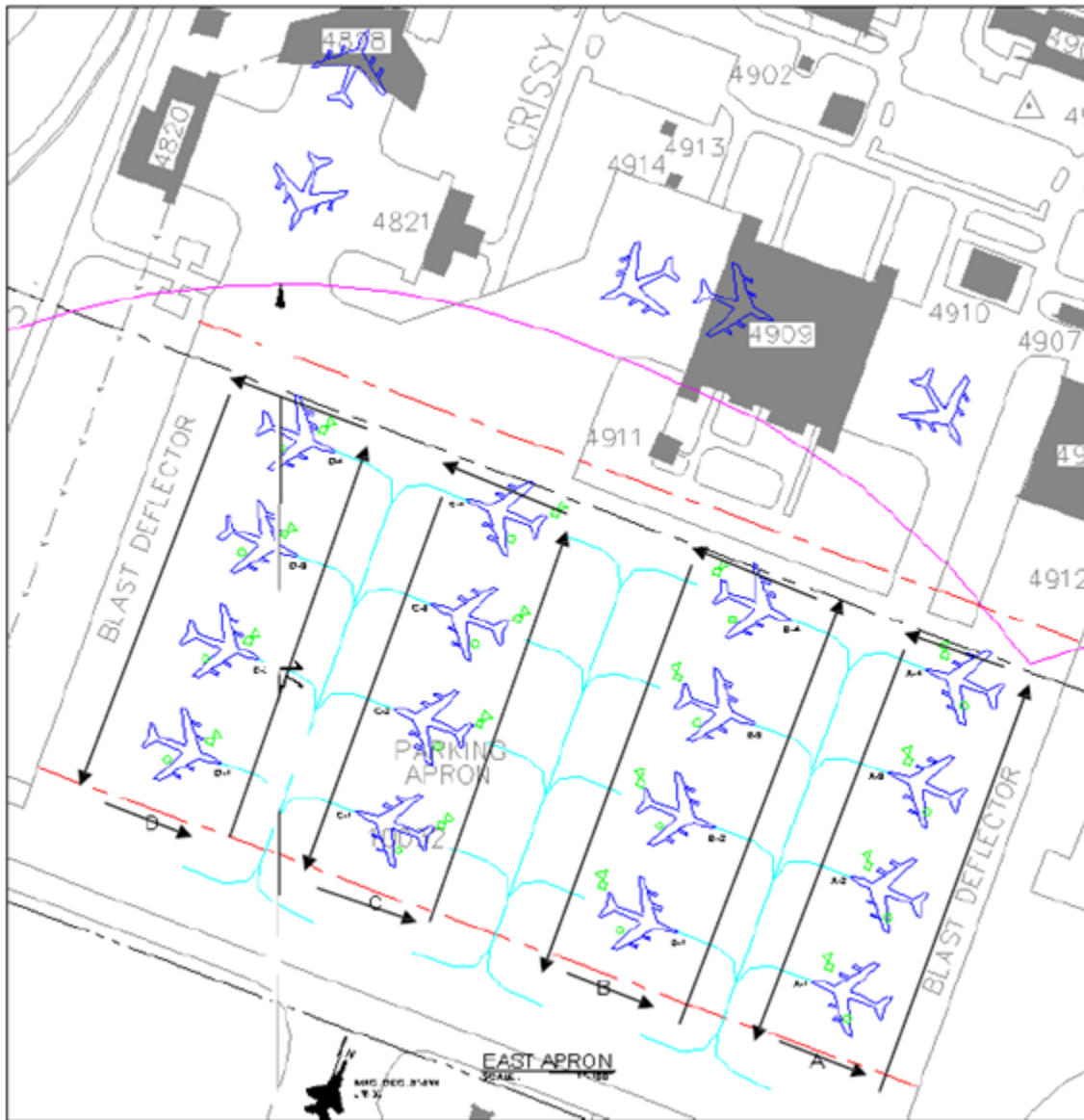
Figure A2.6. Traffic Flow KC-135 Ramp
