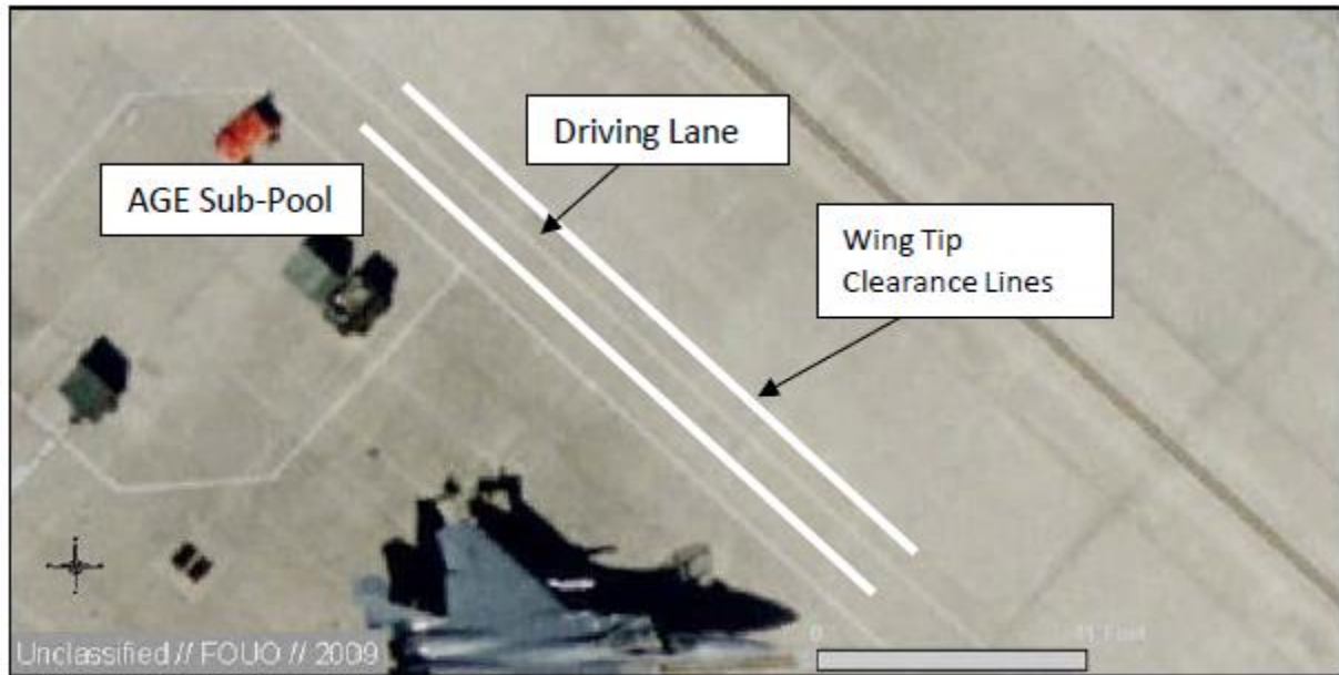
Figure A2.9. Wing Tip Clearance Lines.
