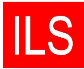
HOLD SIGN AT ILS CRITICAL AREA
