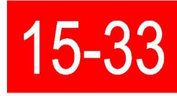
RUNWAY HOLD SIGN (AT INTERMEDIATE INTERSECTION)
