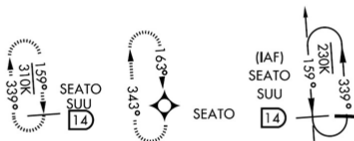
Figure 13.2. Multiple Holding Patterns at Same Fix.
