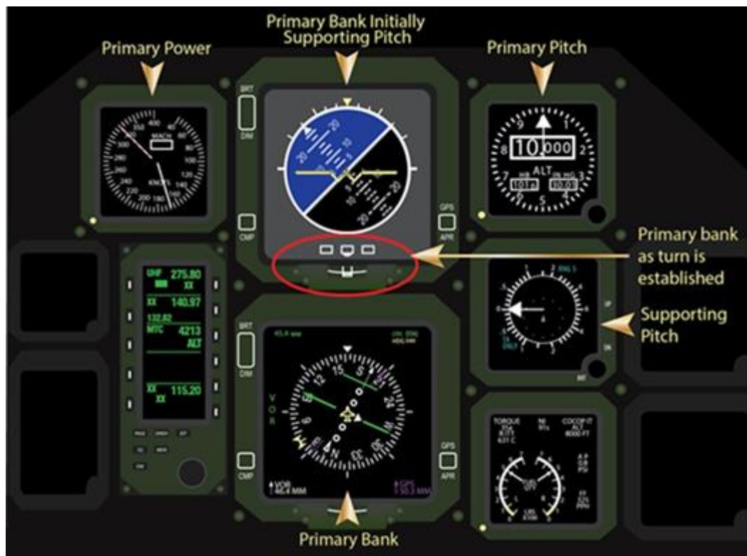
Figure A5.4. Level Turns.
