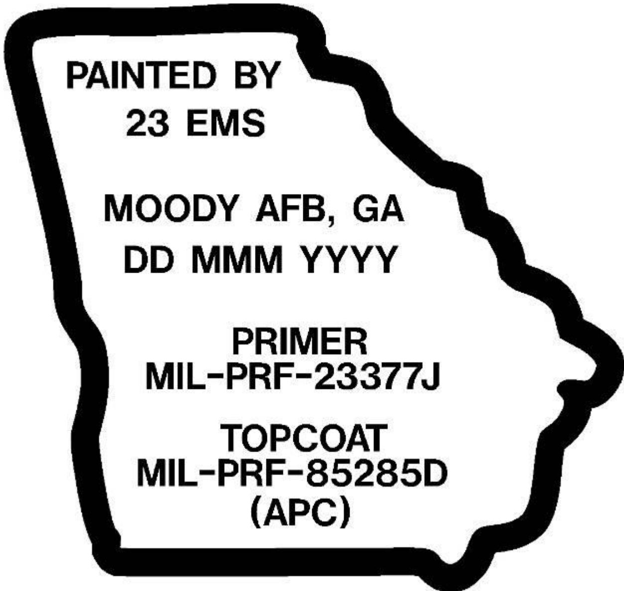
Figure 3.2. (Added) Paint Identification Placard.
