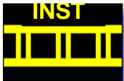
Figure 8.1.9.3.2.1. Runway Instrument (INST) Hold Position Marking
