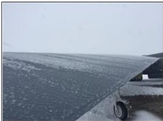
Figure A12.2. (MINOTAFB) De-iced wing with ice crystal contamination present.
