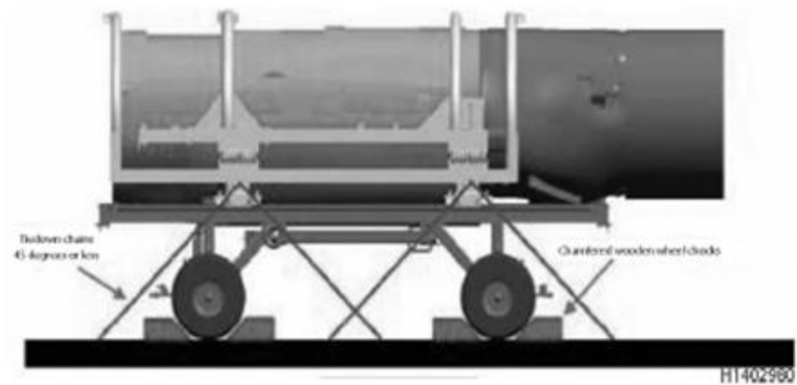
████████ Tie Down and Chock Configuration - View A
