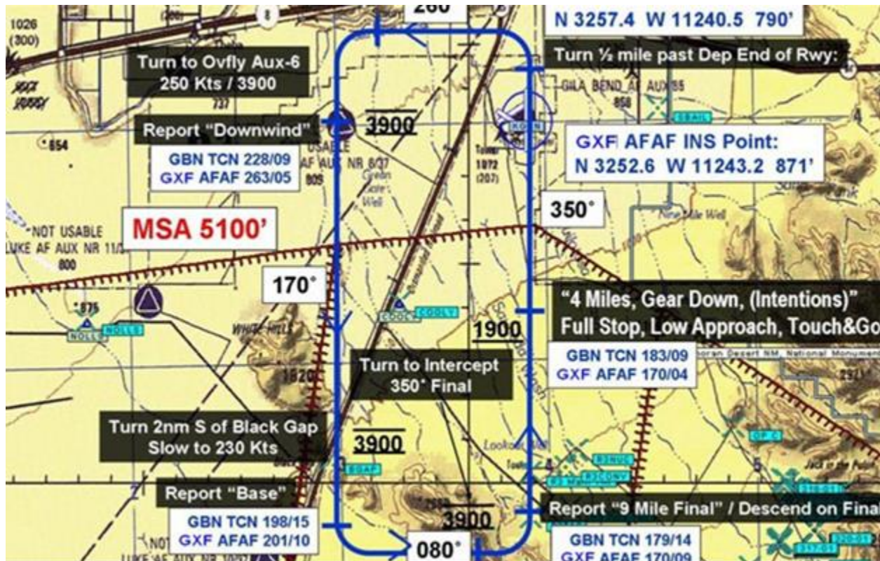
Figure 11.5. GXF Night VFR Straight-in Pattern (NVG Pattern).
