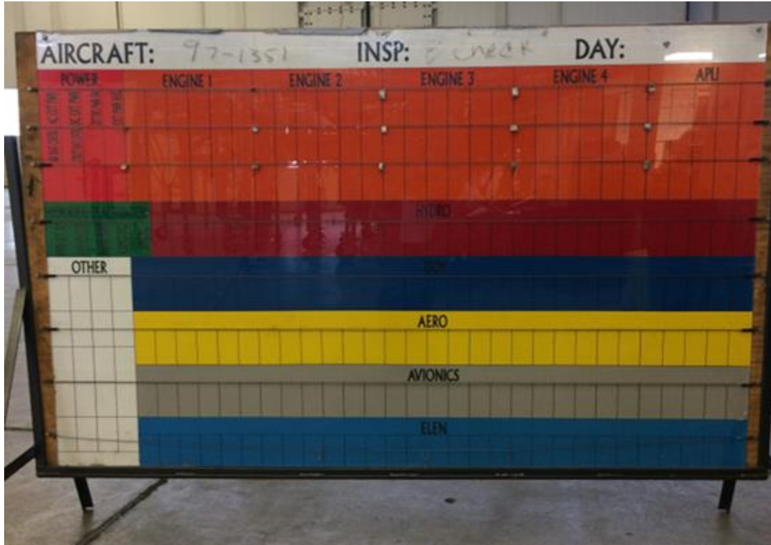
Figure A4.1. Warning Tag Status Board.
