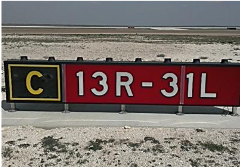
Figure A14.2. (Mandatory) Approach Zone Hold Sign with Location Sign.
