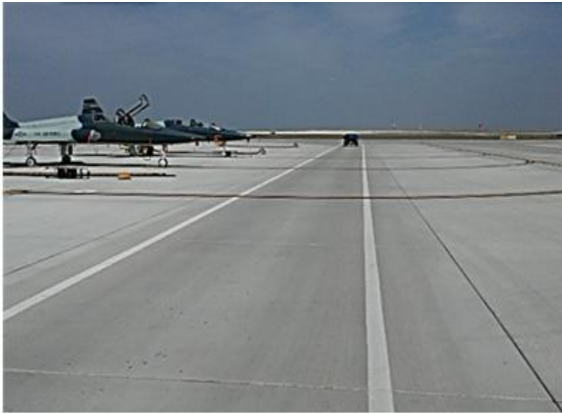
Figure A13.8. Vehicle Stop Bar Marking.
