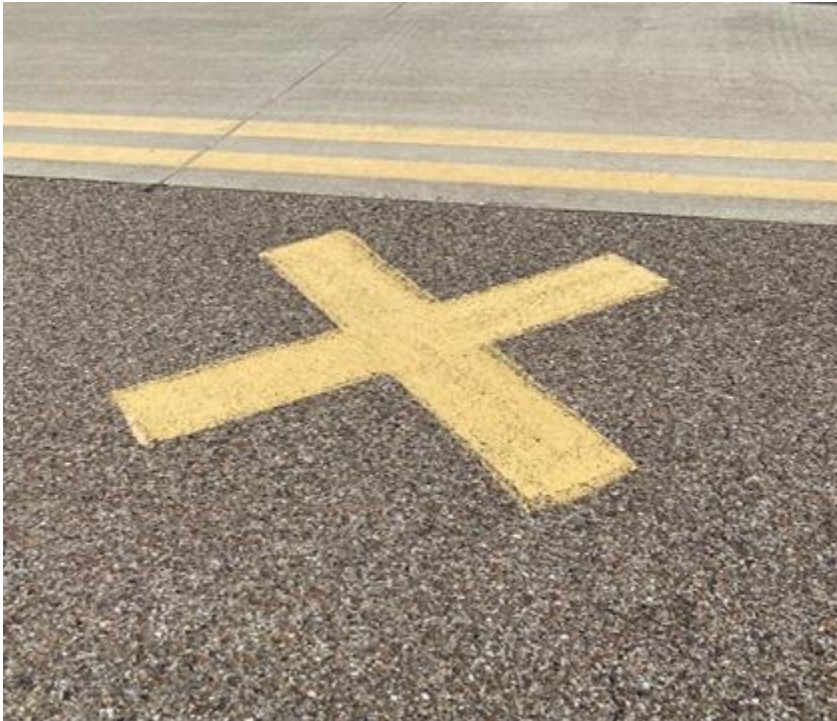
Figure A13.14. Area Closed to Aircraft (Vehicles Only).
