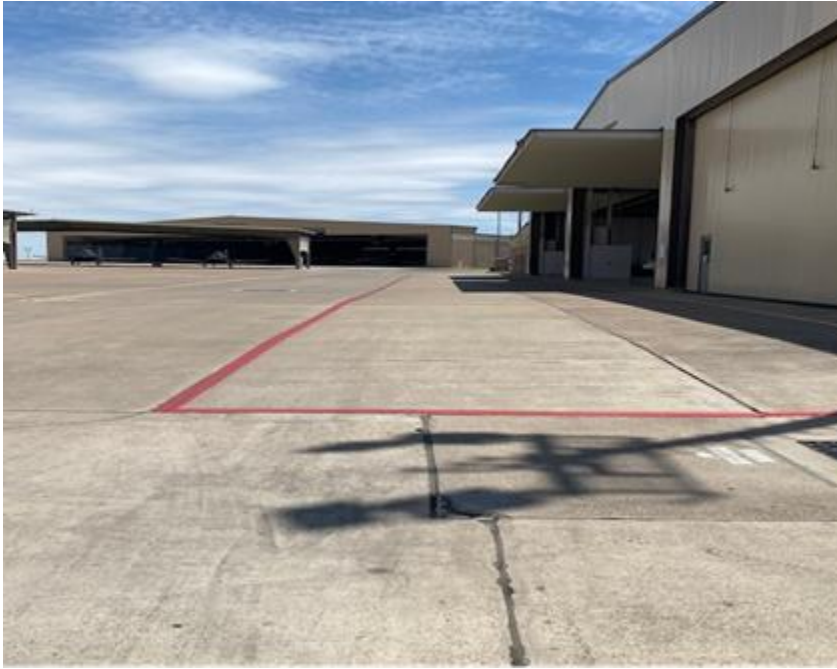
Figure A13.14. Area Closed to Aircraft (Vehicles Only).
