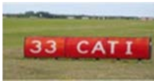
Figure A13.4. Mandatory Instrument Holding Position Sign located at taxiway Mike denotes entrance to area to be protected for an ILS signal or approach airspace.
