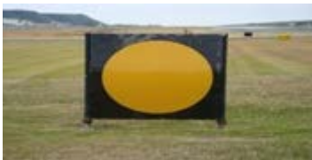
Figure A13.10. Barrier Marker Sign are located North and South of the runway (both sides) and indicates the location of barrier's engagement for fighters.
