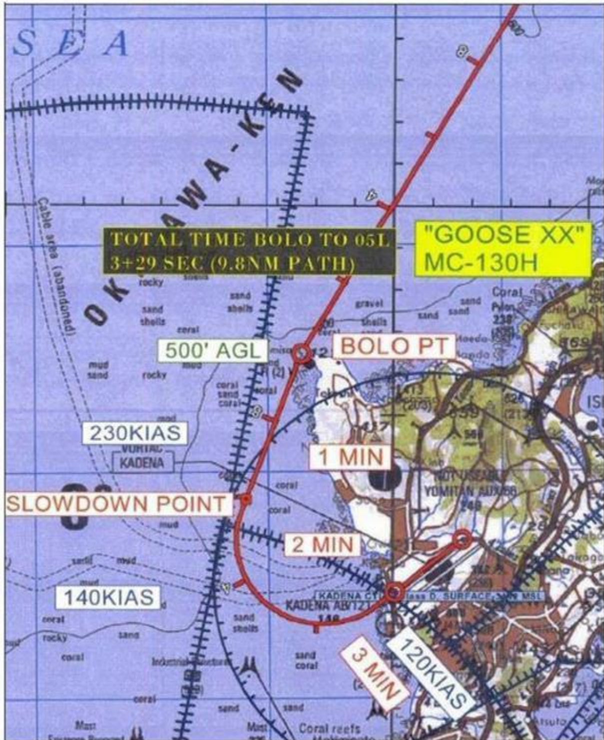
Figure A2.16. Runway 5 Bolo Point SCA for MC-130 Aircraft (GOOSE).
