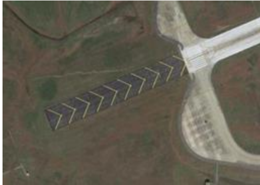
Figure A10.5. FOD Checkpoint Marking and Sign.
