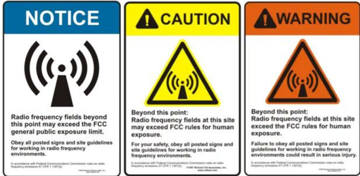
Figure A3.1. Example Appropriate Signs for Hazardous EMFR Areas.
