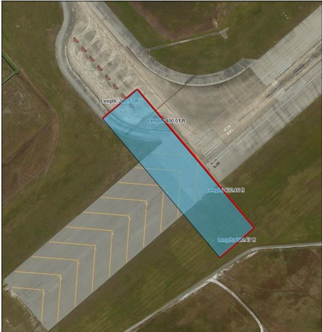
Figure A5.1. Precision Obstacle Free Zone (POFZ).
