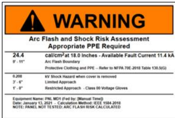
Figure 5.2. Example of Detailed Arc-Flash WARNING Label.
