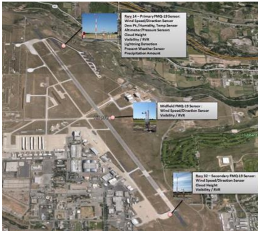
Figure 3.1. Airfield Automated Weather Sensor Locations & Capabilities.
