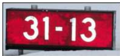
Figure 6.1. Runway Hold Sign.
