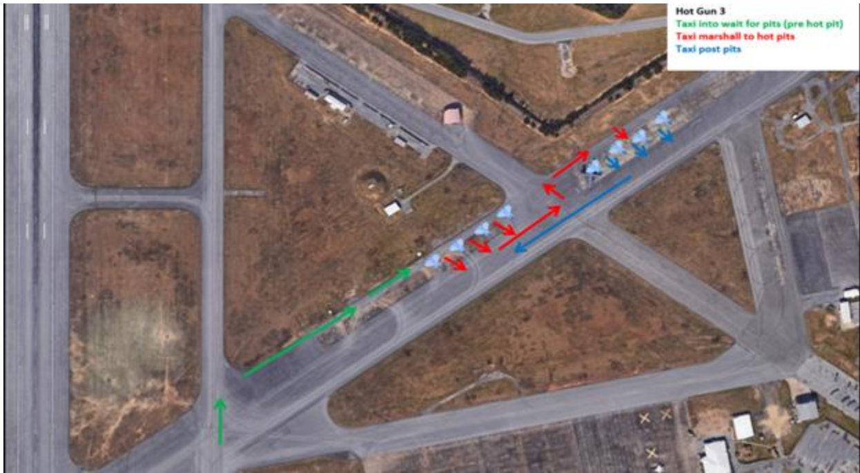
Figure A2.5. Eglin AFB HG3 Hot Pits.
