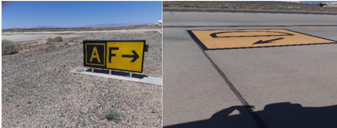
Figure 4.5. (Added-EDWARDSAFB) . Taxiway Location Sign.
