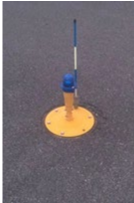
Figure A13.2. High Intensity Runway Light.
