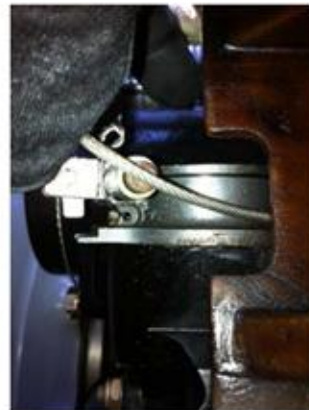
Safety Wire Hole On Sump Filler Cap
