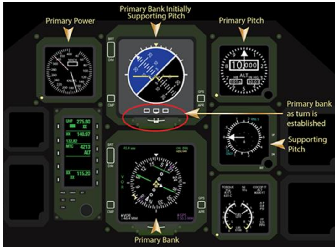
Figure A5.4. Level Turns.
