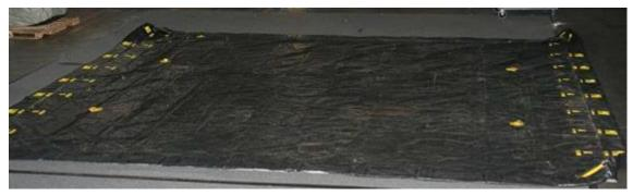
**Step 4.** Move the shelter bag to the center of the berm (**Figure A3.7**.). This step requires four people. Use the lifting straps located on the bag to move the shelter. Team members should lift high and avoid dragging the shelter. Assuming the shelter was packed correctly, the top should have yellow reflectors indicating the direction of the shelter throughput (**Figure A3.8**).
