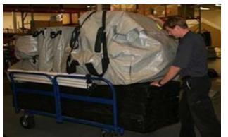
**Step 2.** Remove the berm from the berm bag (**Figure A3.5**).
