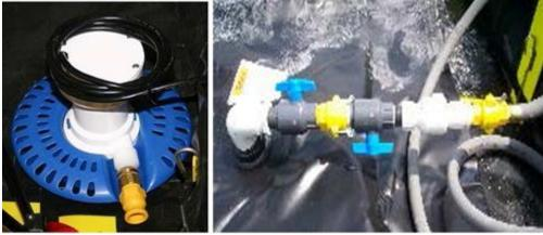
Step 4. Ensure GFCI protection, and plug the pump into a 110-volt outlet.
