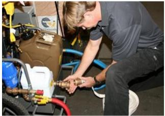
**Step 7.** Before starting the water heater, ensure that the fuel can contains diesel fuel (NOT biodiesel) and that 110-volt GFCI protected electricity is available. **Note:** Follow manufacturer's instructions.
