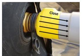
**Note:** The pressure relief valve opens at 4 PSI and self-resets (closes) at 3.5 PSI. This means that when the valve is opened, air will escape for some time until the lower pressure of 3.5 PSI is reached. The electric pump will not cause over inflation, but deployment with air bottles may cause damage, so ensure the pressure relief valves are clear of debris.
