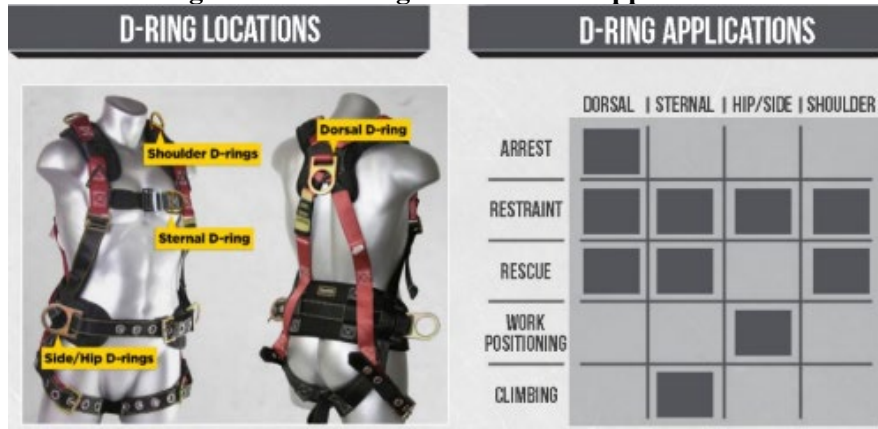
Figure 12.2. D-Ring Location and Application
