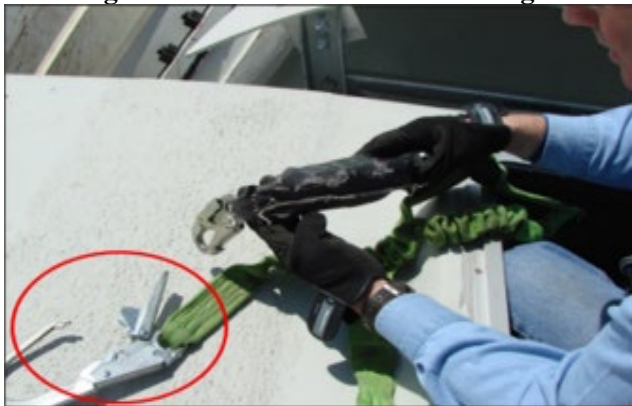
Figure 16.2. Forced Roll Out Damage.
