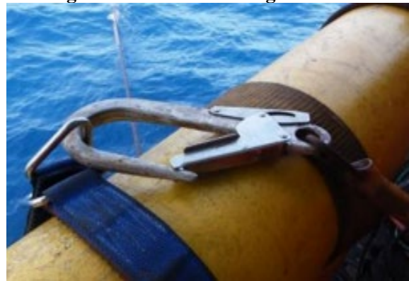
Figure 16.3. Side Loading Hazard.
