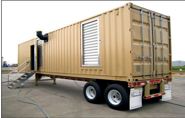
Figure 7.8. Interim Power Unit (IPU)
