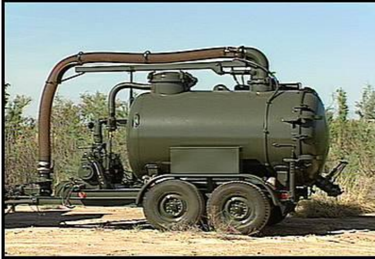
Figure 9.2. Wastewater Disposal Trailer
