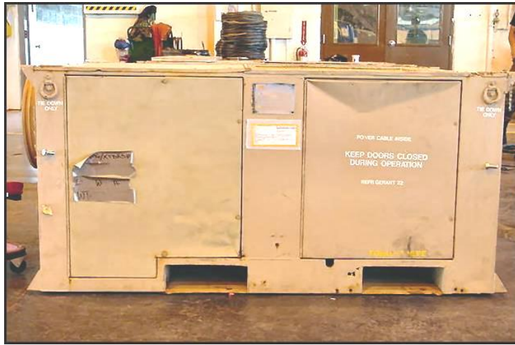
Figure 11.12. A/E32C-39 Environmental Control Unit
