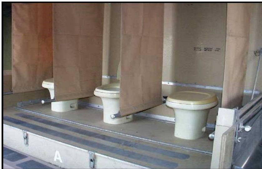
Figure 10.15. Field Deployable Latrine
