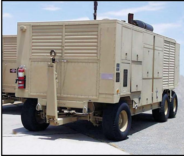
Figure 7.6. MEP-012A 750-kW Generator
