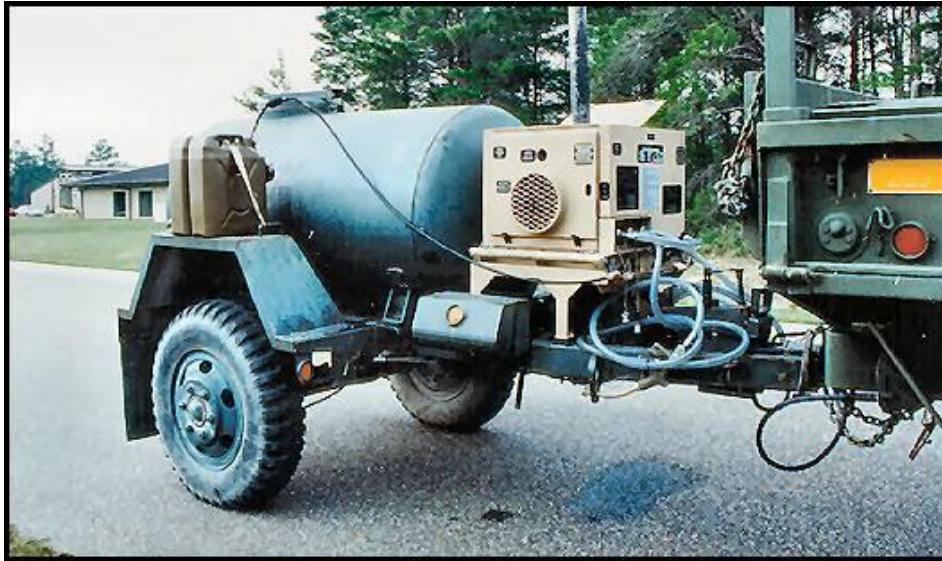
Figure 8.7. 400-Gallon “Water Buffalo” Trailer With Chiller Attached
