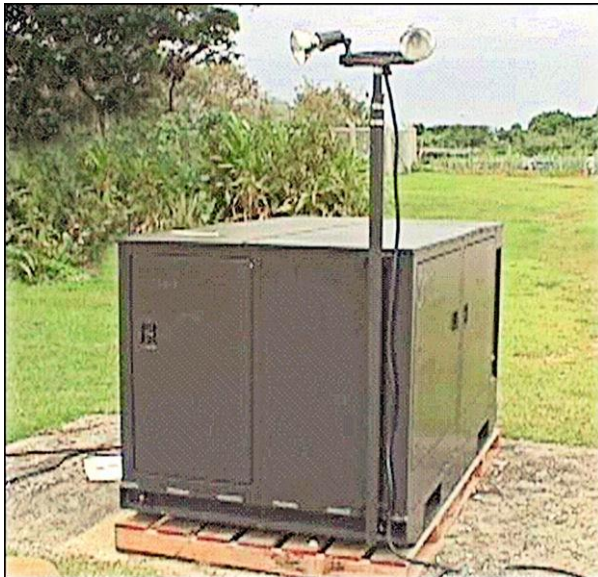
Figure 7.10. Remote Area Lighting System (RALS)
