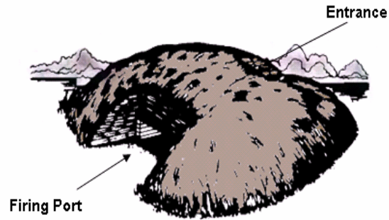
Figure 3.3. Top View – Fighting Bunker.
