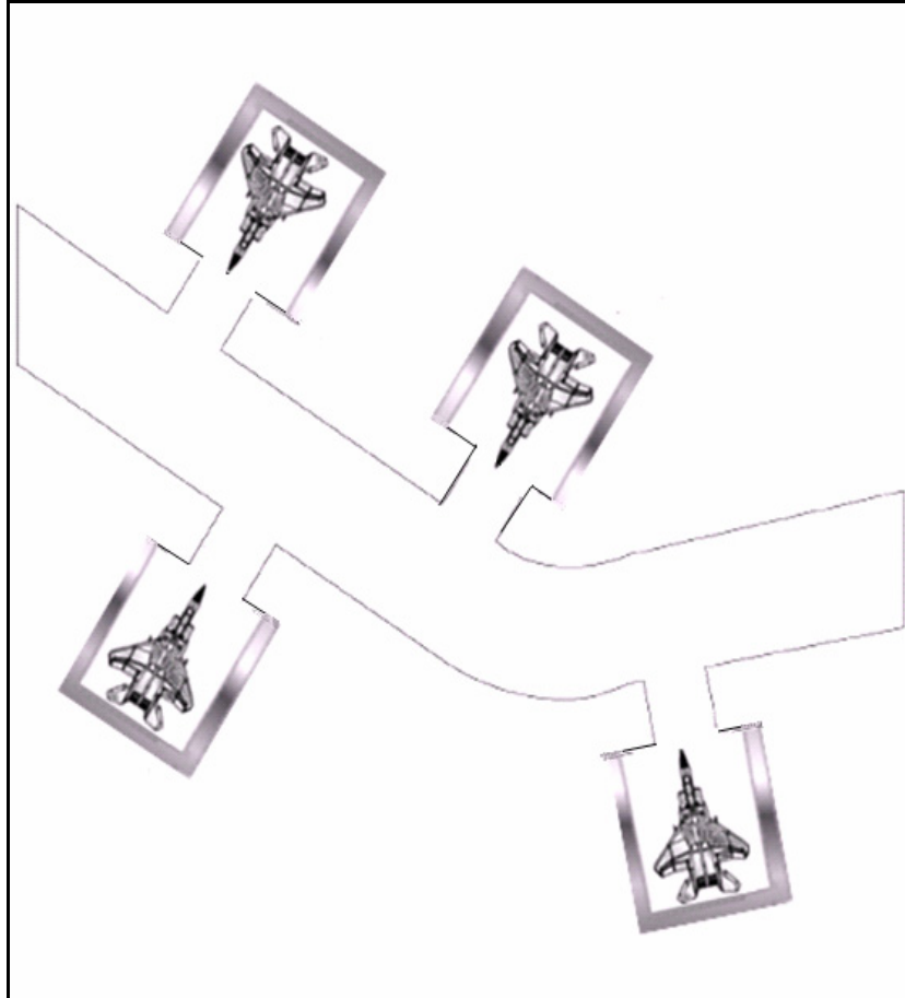
Figure 5.29. Dispersed Pattern for Aircraft Revetments.
