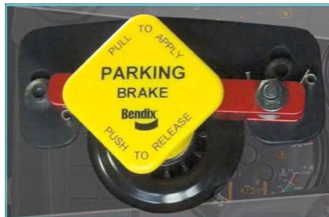
Figure 2.28 Parking brake panel
