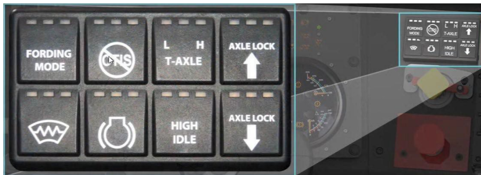
Figure 2.30 Systems control multiplexed switch panel
