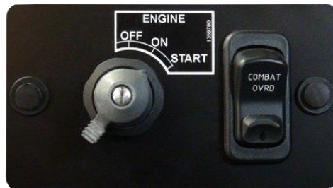
Figure 3.3 Ignition switch panel
