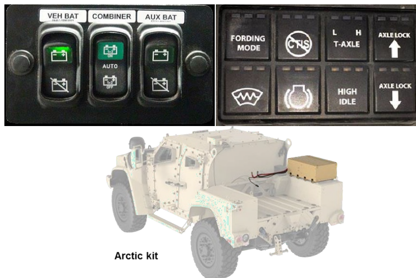
Figure 3.7 Operating in extreme cold conditions
