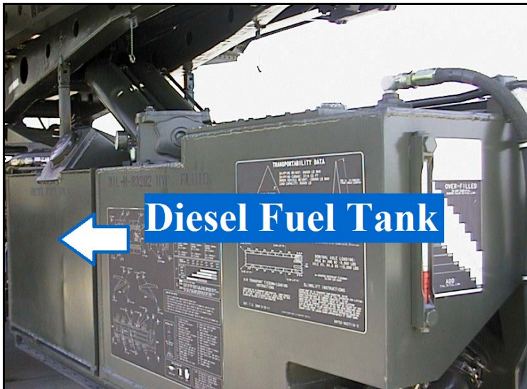
Figure 5.3. Diesel Fuel Tank.
