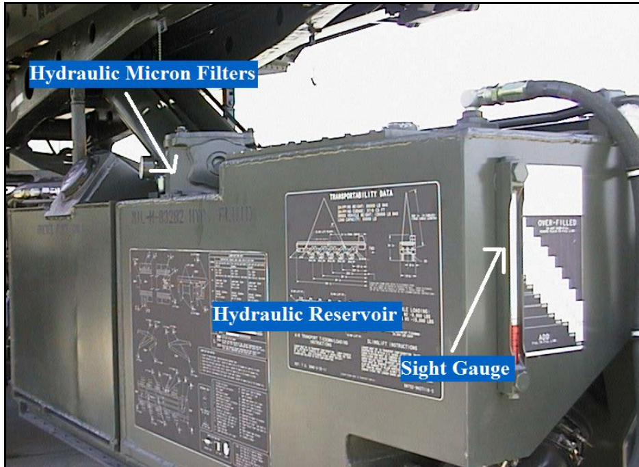
Figure 5.5. Hydrostatic Drive Hydraulic System.
