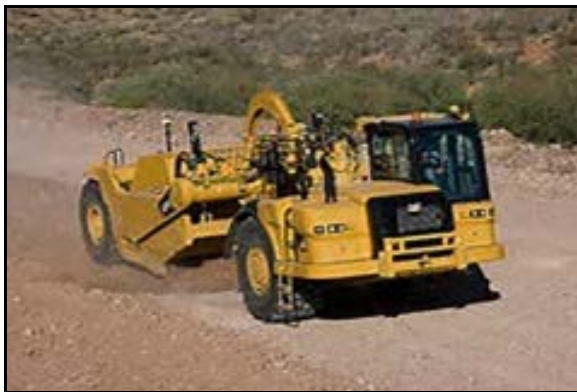
Figure 5.3. Dumping and spreading.
