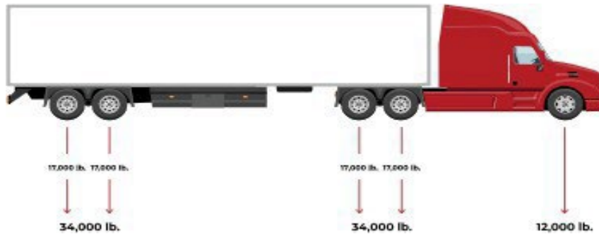
Figure 4.1. Axle Load Distribution.
