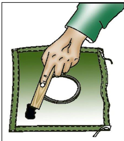
Figure 4.44. Repairing Small Hole in Stovepipe Shield.
