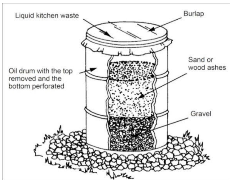
Figure 4.28. Barrel-Filter Grease Trap.
