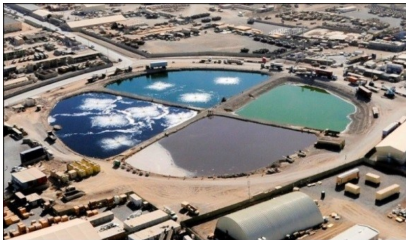
Figure 4.19. Lagoon System with Several Cells.
