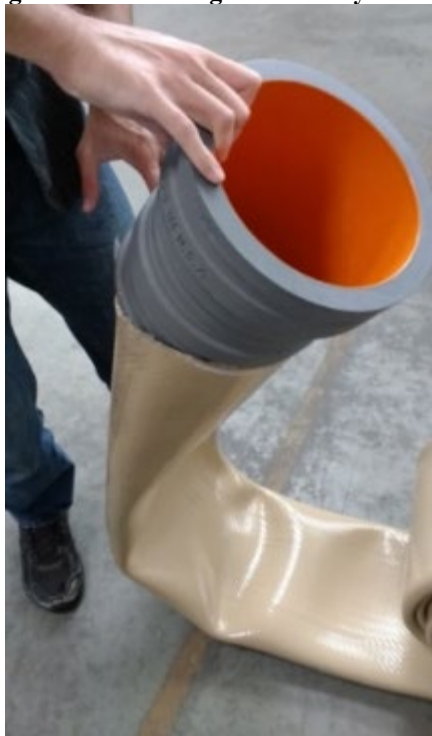
Figure 4.5. Inserting Hose End Fitting into the Layflat Hose End
