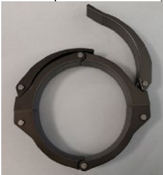
Figure 4.15. First Lever Clamped and Second Lever Partially Clamped.
