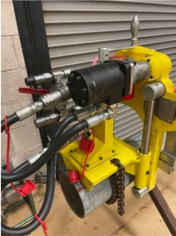
Figure 2.10. Tightening the Drive Adapter Screw.
