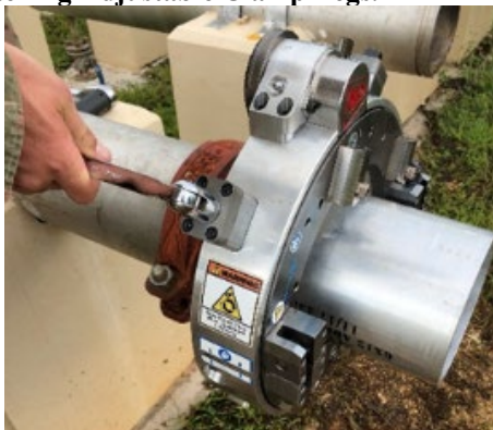
Figure 2.33. Tightening Adjustable Clamp Legs.
