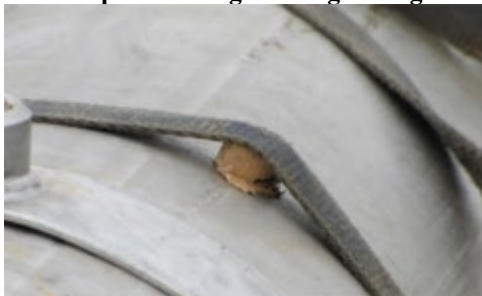
Figure 3.16. Ratchet Strap Increasing Holding Strength of Wood Plugs.
