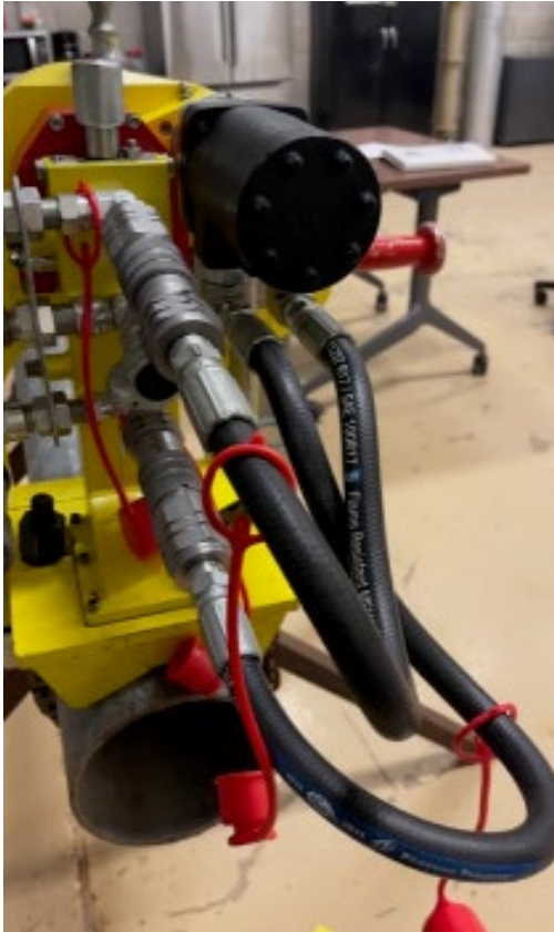
Figure 2.11. Hydraulic Motor Installed on Saw.
