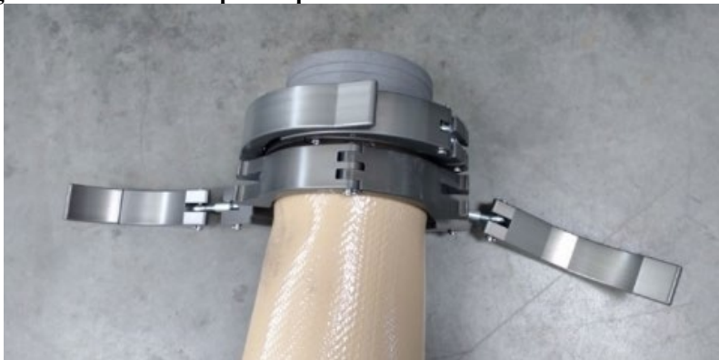
Figure 4.17. Second Snap Clamp Placement.
