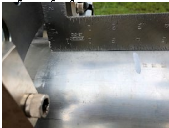
Figure 2.32. Placing Rotating Ring 3.75 Inches from Cut Line.
