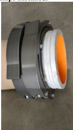
Figure 4.18. Both Snap Clamps Installed.
