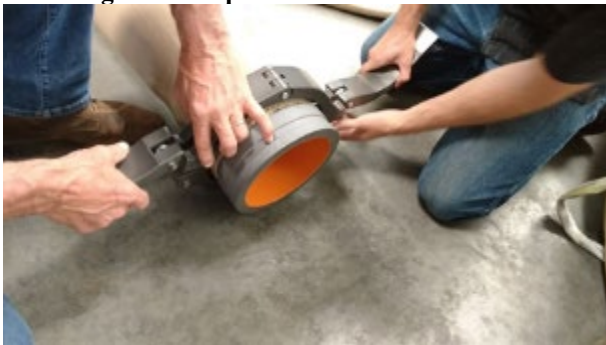
Figure 4.14. Hooking the Clamp Levers in the Notches.
