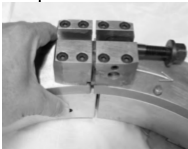
Figure 2.55. Ring Halves Separation.
