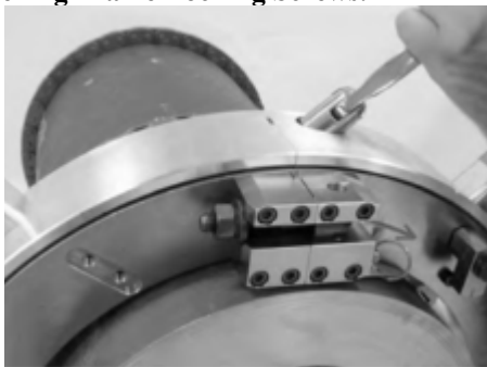
Figure 2.60. Tightening Frame Locking Screws.
