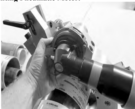
Figure 2.47. Mounting Pneumatic Motor.
