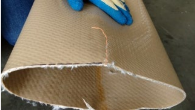
Figure 4.3. Layflat Hose with Bonding Wire Exposed.
