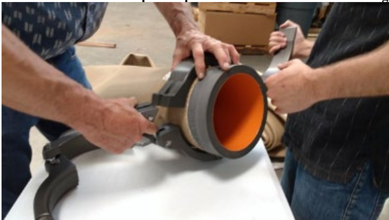
Figure 4.12. Position the Snap Clamp on the Installed Hose End Fitting.
