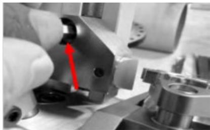
Figure 2.45. Tightening Trip Position Screw after Aligning Trip to the Star-Wheel.
