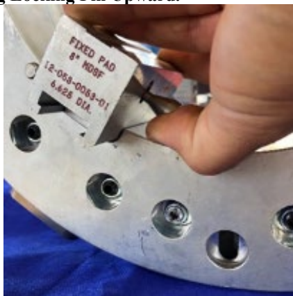
Figure 2.30. Pulling Locking Pin Upward.
