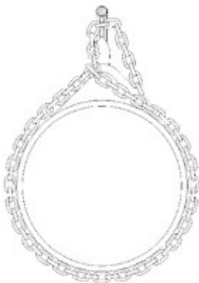
Figure 2.66. Chain Lassoed Around Pipe & Connected to Alignment Bar Chain Hook.
