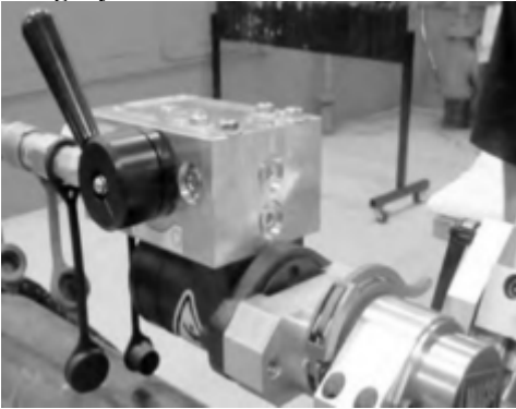
Figure 2.48. Mounting Hydraulic Motor.
