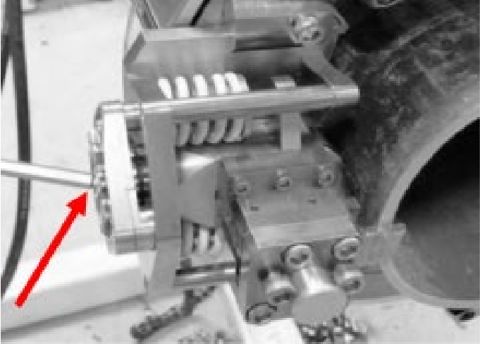
Figure 2.51. Parting/Grooving Slide Adjustment.
