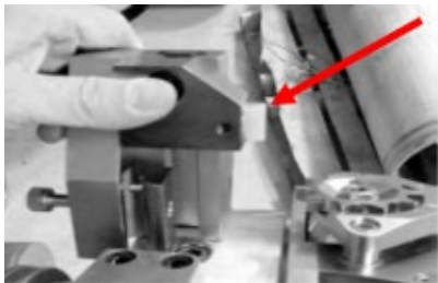
Figure 2.43. Aligning Base of Trip Assembly & Tightening Trip Mounting Screw.
