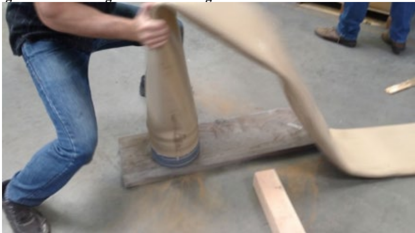
Figure 4.6. Installing Hose End Fitting.
