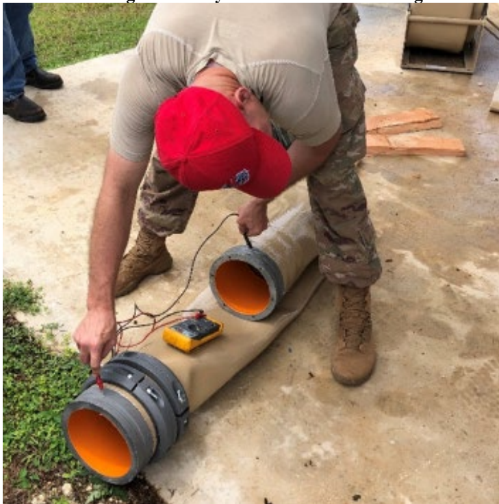
Figure 4.8. Performing Continuity Test on Hose End Fittings.
