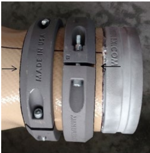
Figure 4.11. Completed OEM Hose End with Both Clamps Installed and Lines Drawn.
