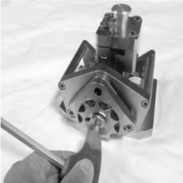
Figure 2.35. Turning Star-Wheel to Retract the Slide.
