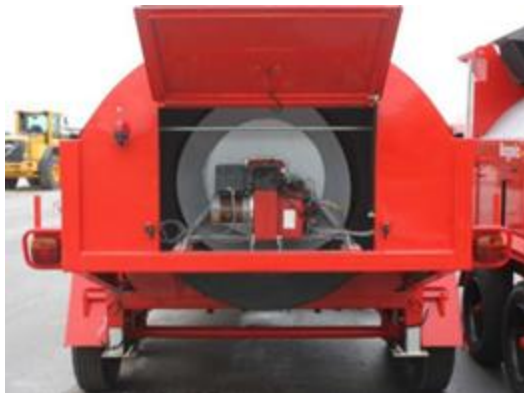
Figure 1.4. Asphalt Recycler Burner (Rear Hatch).
