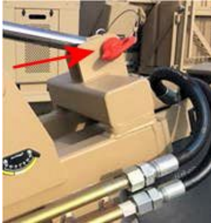
Figure A4.17. Hoist Cylinder Pinned to Mounting Holes.
