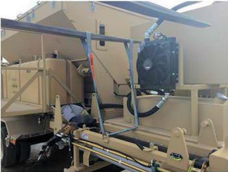
Figure A4.14. Lifting Spare Mixer Assembly from Storage Location.
