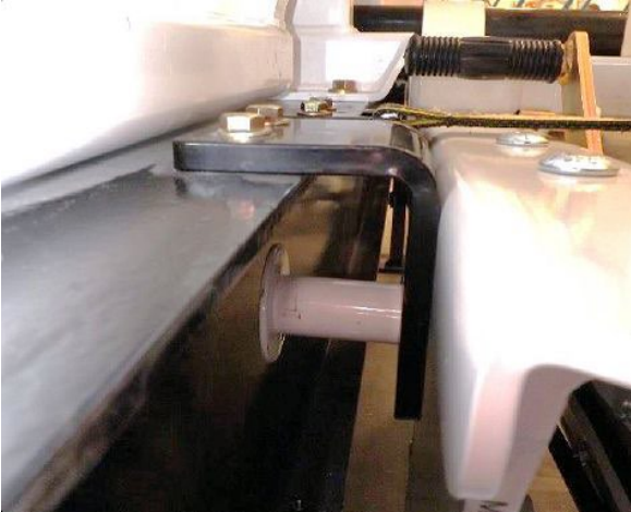
Figure A4.7. Front Auger Holding Bracket.
