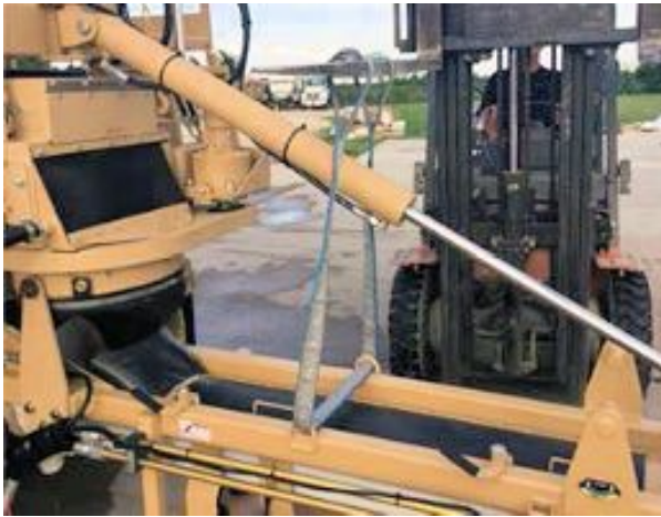
Figure A4.9. Lifting Mixer to Relieve Pressure on Cylinder.
