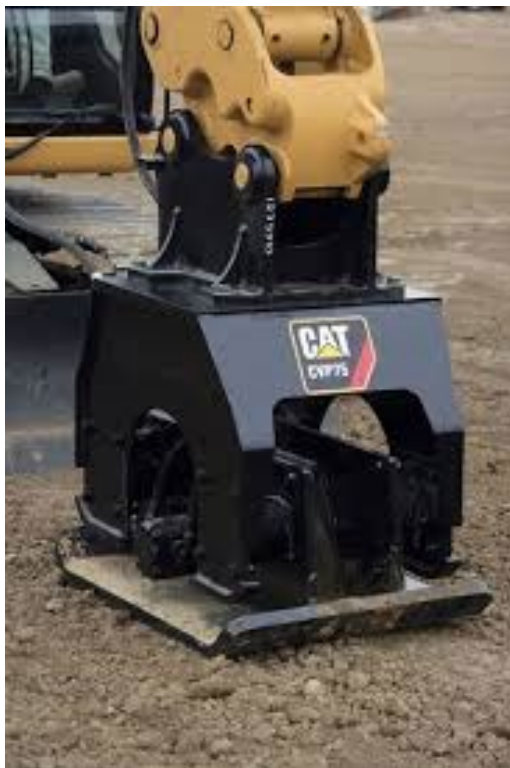
Figure 5.6. Excavator with Plate Compactor Attachment.
