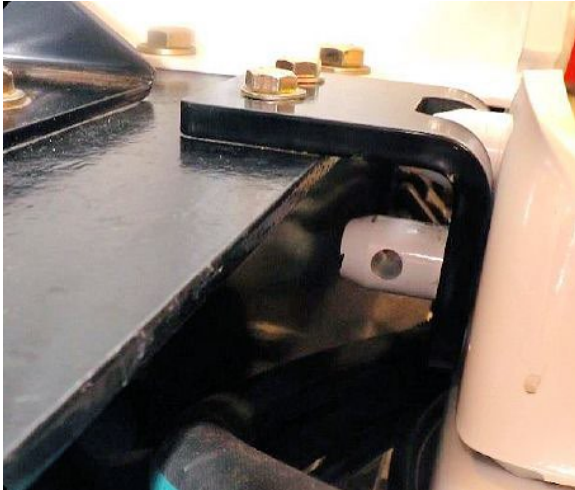
Figure A4.6. Rear Auger Holding Bracket.
