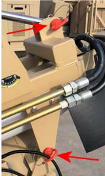
Figure A4.10. Pins Holding Cylinder and First Chute from Mixer Assembly.
