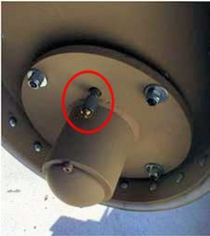
Figure A4.19. Area Where Grease Will Exit the Seal.
