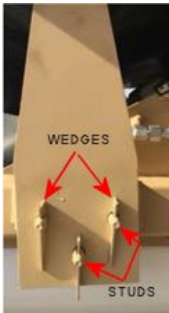
Figure A4.13. Retaining Wedges and Arm Studs.
