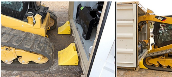
Figure 2.25. Wheel Chocks in place to Prevent Connection Block Damage.
