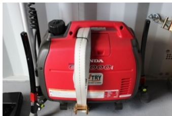
Figure 2.15. Generator for Telescoping Area Lighting.
