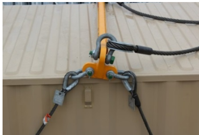
Figure 2.10. Slings Connected to Spreader Bar.
