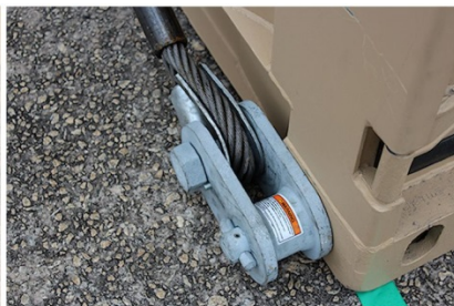
LIFTING LUG INSERTED AND LOCKED
