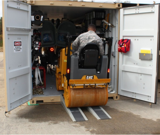
Figure 2.24. Roller Backing Down Ramps.
