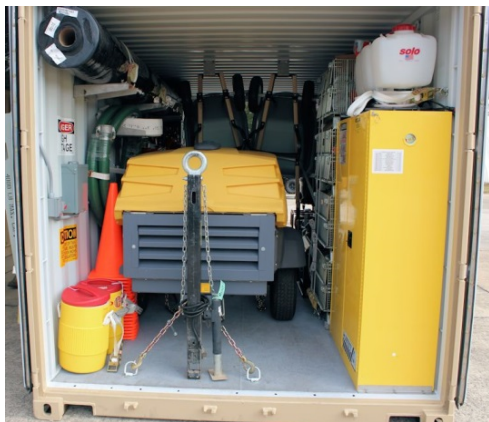
Figure 2.14. Flammable Storage Cabinet.
