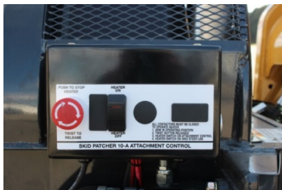
Figure 2.40. Asphalt Heater Red Emergency Stop Button.
