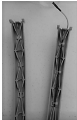
Figure 7.18. Non-Antenna and Antenna Legs.
