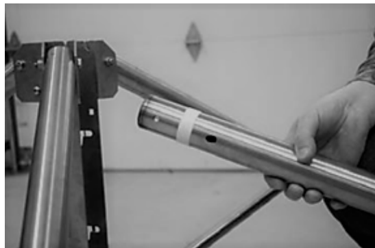
Figure 7.6. Identification of the Bottom Section with Welded Stiffener Tube.
