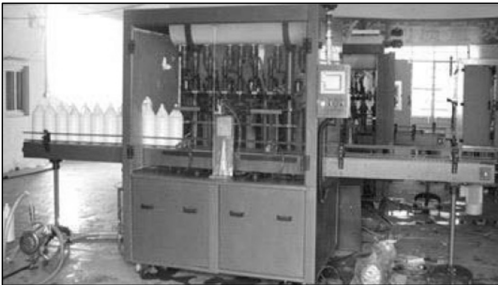
Figure G-2. Example of chemical filling equipment
