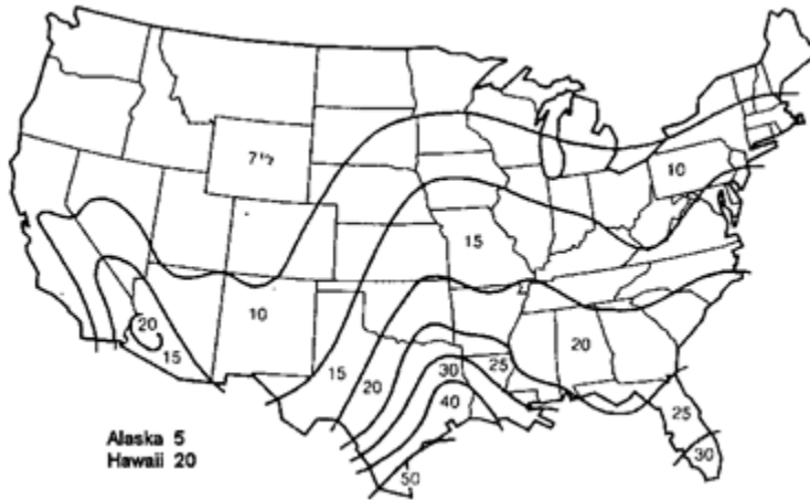
Figure 4.5. Required Ventilation to Control Temperature.
