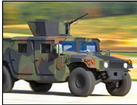
Figure 3.7. HMMWV with Pattern Paint Applied.
