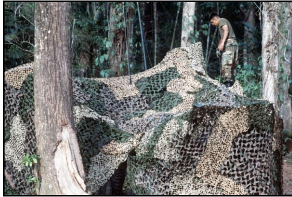
Figure 3.4. Placing Netting over Vehicle to Blend with Background.
