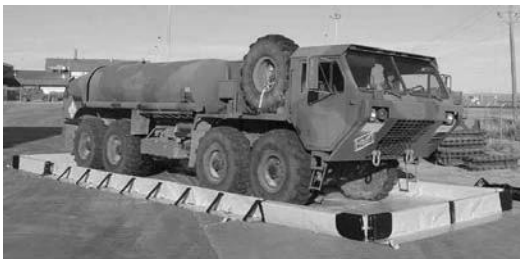
Figure 3.5. Secondary Containment for Refueling Vehicle.
