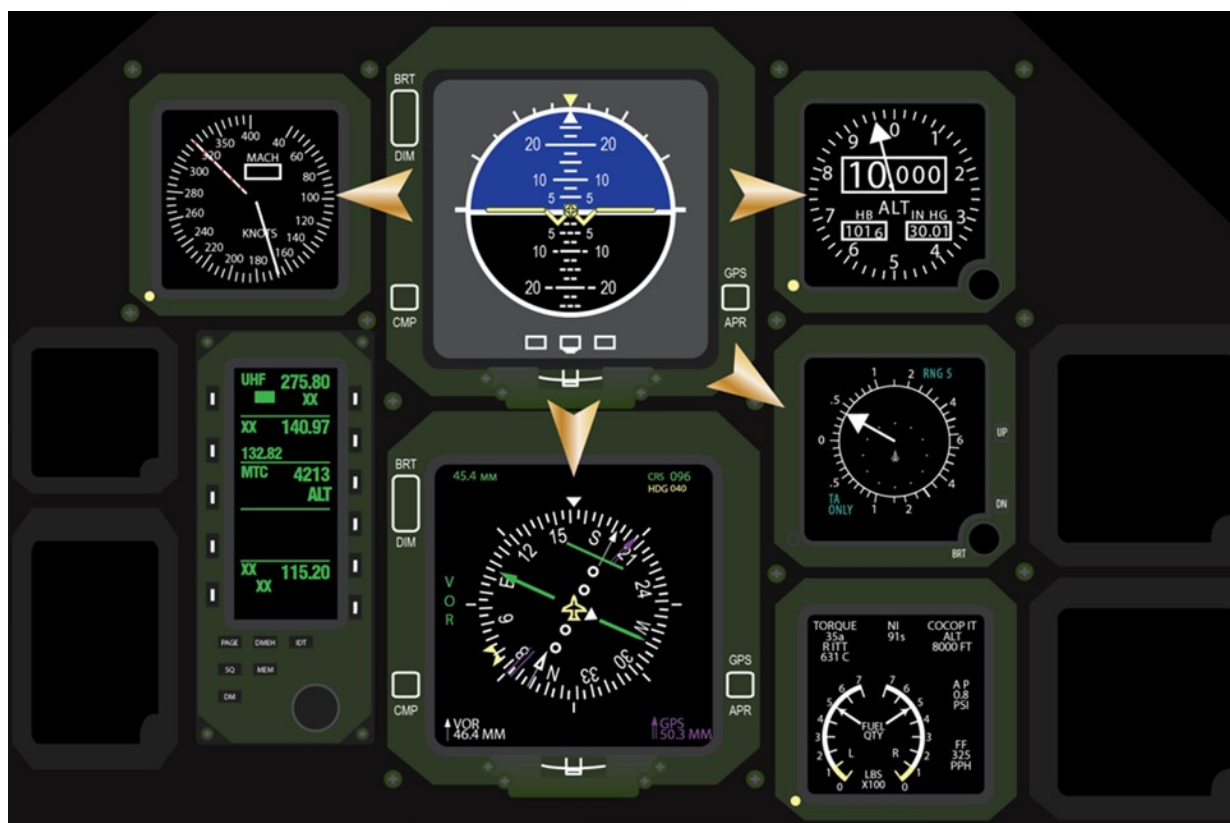
Figure A4.4. “Hub and Spoke” Cross-check.
