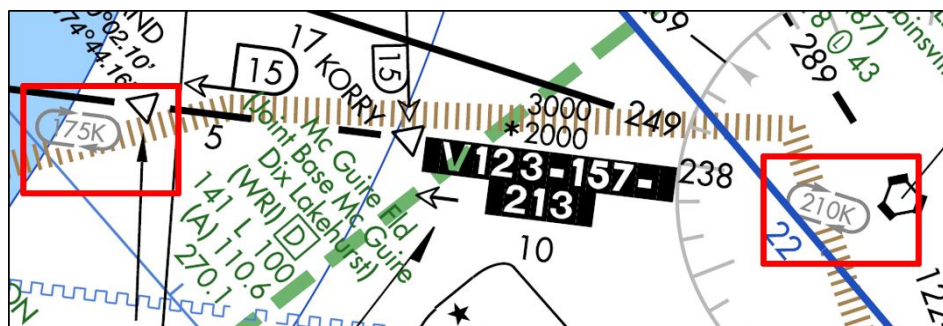
Figure 13.4. Maximum Holding Airspeed.
