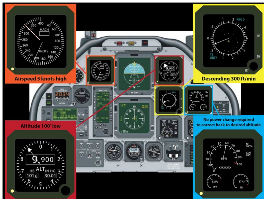
Figure A5.3. Airspeed Deviation.
